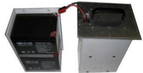
Figure 6 Uncovered and enclosed battery packs
