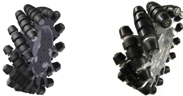
Figure 4 Mecanum Wheels (a) CAD Design (b) Final Product
