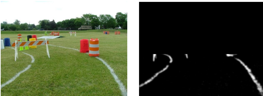
Figure 11 Lane Detection: (a) from camera (b) post processing
